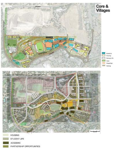
Remediation of the landfill not only results in an additional 36 acres for facilities development and 36 acres for low-intensity uses such as surface parking, athletic fields and solar power the landfill to fill and grade the pumice mine, rather than having to import material from off-site.
